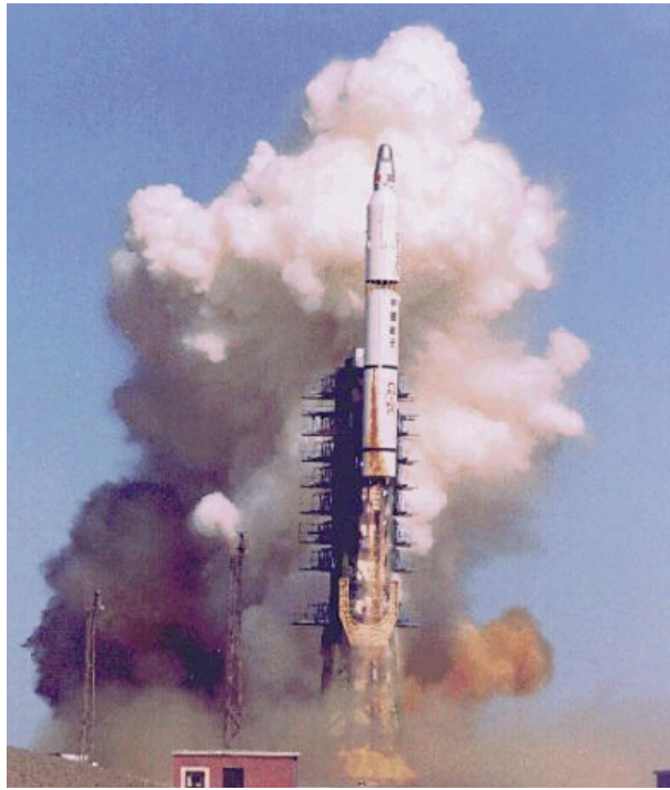
The Long March 2E (far left), carrying Hughes satellites, crashed in 1992 and 1995. In the aftermath of those crashes, Hughes engineers worked with the PRC to improve the rocket's fairing, which had twice ripped apart under launch conditions. The Long March 2E uses a stretched version of the Long March 2C (left), increasing the burn-time of the engines and adding four boosters.
